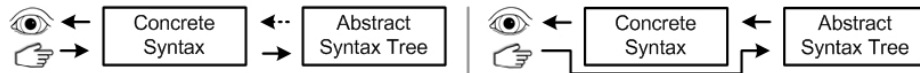
Fig. 1. In ParEs (left), users see and modify the concrete syntax. A parser constructs the AST. In ProjEs, users see and interact with the concrete syntax, but changes directly affect the AST. The concrete syntax is projected from the changing AST.
