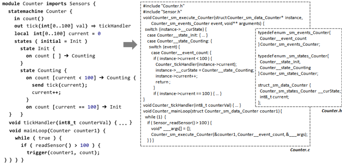
Figure 8. A state machine is embedded in a C module as a top level construct. It declares in and out events as well as local variables, states and transitions. Transitions react to in events, and out events can be fired in actions. Through bindings (e.g. tickHandler ), state machines interact with C code. State machines can be instantiated. They are transformed to enums for states and events, and a function that executed the state machine using switch statements. The trigger statement injects events into a state machine instance by calling the state machine function.
